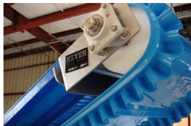
Polymer standoff bearings with stainless steel inserts.
